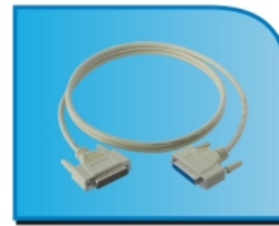
XYC005 SERIAL CABLE DB25M/DB25M MOLD XYC007 SERIAL CABLE DB25M/DB25F MOLD XYC009 SERIAL CABLE DB25F/DB25F MOLD
