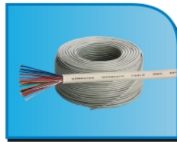
XYD014 2464 SINGLE SHIELD COMPUTER CABLE RATING:80℃ 300V SPECIFICATION:28AWG SHIELD:AOL SHEATH:PVC REEL:100M CONDUCTOR:4,5,6,9,15,18,25
