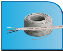
XYD018 USB CABLE RATING:80℃ 300V SPECIFICATION:2C/28AWG AND 2C/26AWG SHIELD:AOL+COPPER BRAID SHEATH:PVC REEL:100M
