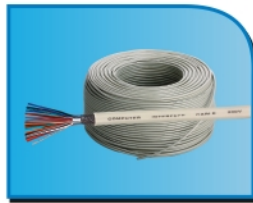
XYD015 2464 DUAL SHIELD COMPUTER CABLE RATING:80℃ 300V SPECIFICATION:28AWG SHIELD:AOL+BRAID SHEATH:PVC REEL:100M CONDUCTOR:4,5,6,9,15,18,25
